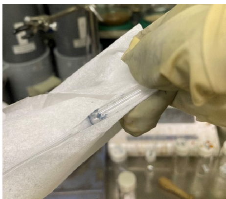
Figure S2. 'Stained' solid on filter (presumably KI) after rinsing with chlorobenzene.
