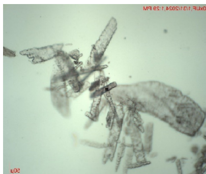
Figure S5. Crystals of [\text{Pu}_2(\text{tBu-PDB})_6] used to acquire solid-state UV-vis-NIR data. The black square indicates where the area of the crystal that was probed by the CRAIC spectrophotometer.
