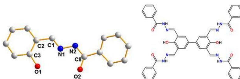
Supplementary Figure 7. The crystal structure of monomer model N' -(2-Hydroxybenzylidene)benzohydrazide and the structure of monomer model N',N'',N''',N'''' -((1E,1'E,1''E,1'''E)-(4,4'-dihydroxy-[1,1'- biphenyl]-3,3',5,5'- tetrayl) tetrakis (methanylidene)) tetra (benzohydrazide).
