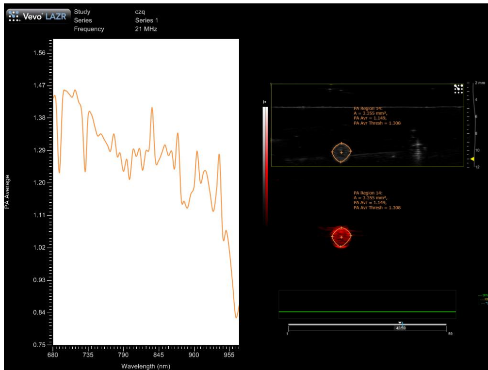
Figure S19. The PA signal changes of PFNB-NC siRNA irradiated by a laser at full spectrum ranging from 680 to 950 nm, and the peak appeared at 690 nm.
