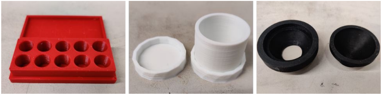
Figure S1: 3D-printed PLA molds for casting the materials into the desired shape.
