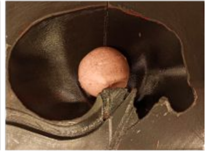
⑨ Place the PVC skeleton in torso mold
