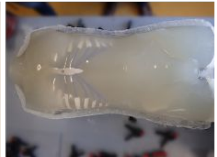
⑫ Prepared torso phantom with organs
