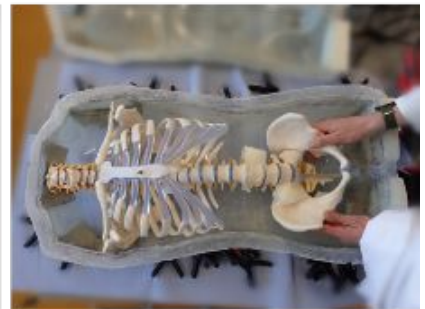
⑫ Prepared torso phantom with organs
