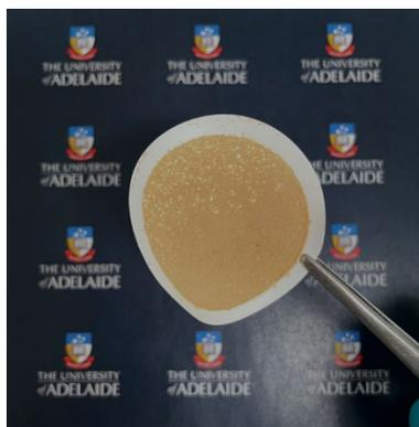
**Supplementary Fig. 32 | Catalysts after reaction.** FeSA-hCN catalysts collected after hydrothermal treatment. Reaction conditions: [UHMWPE MPs] = 1 g L<sup>-1</sup>, [catalysts] = 1 g L<sup>-1</sup>, [H<sub>2</sub>O<sub>2</sub>] = 100 mM, hydrothermal temperature = 140 °C and neutral pH.
