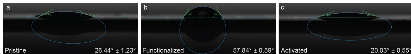
Figure S12: Contact angle measurement images of membrane chip surface. a) Before functionalization, b) after functionalization, and c) after end group activation with NHS/EDC. For each case, twenty measurements were performed, and the corresponding average contact angle and its standard deviation are indicated on the bottom right.
