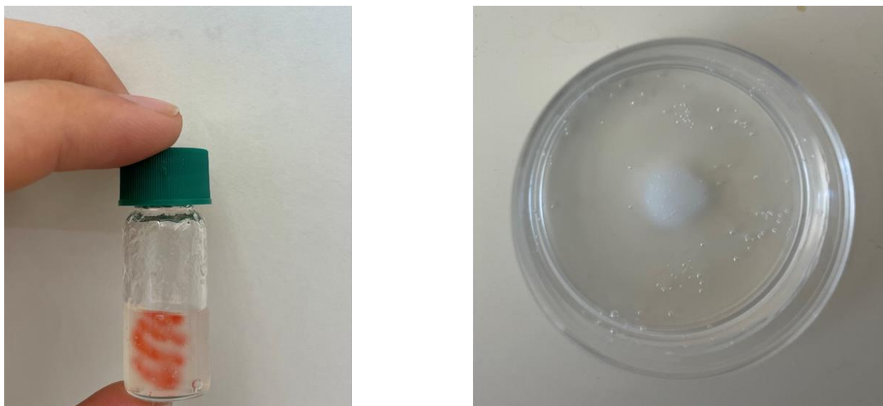
Figure S5. Illustration of 3D Printing a spiral inside the silk bath using the red dye colored collagen solution (left) and printing a disk inside the silk bath using the CH solution (right, the bioink turned white at 37°C).
