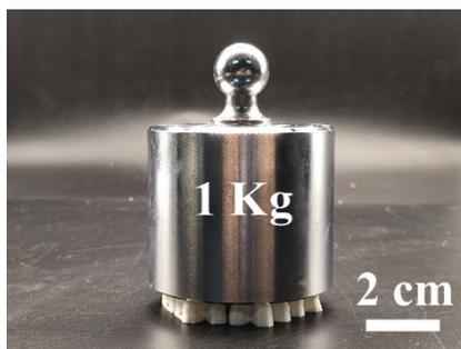
**Figure S16.** Photograph showing 4%-KNF-PVA aerogel withstanding the compression from 1 Kg weight.
