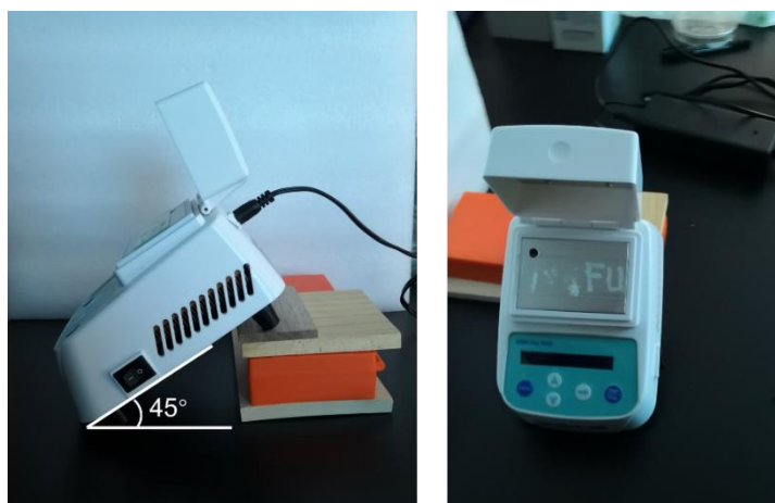
Figure S10. The photos of the patterned glass slide on a heating plate with a tilt angle of 45^\circ for the imaging test. The patterned letters of “NE” are formed by stearic acid, and the letters of “FU” are formed by C18-UCNCs.
