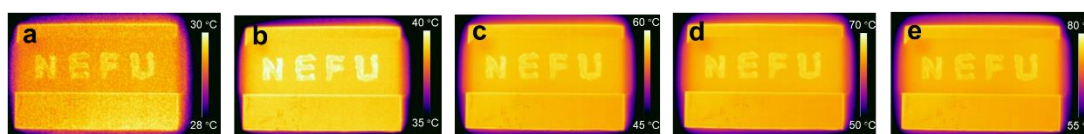
Figure S9. (a-e) Infrared images showing the temperature variations of the patterned glass slide on a heating plate at different set temperatures of (a) 30 °C, (b) 40 °C, (c) 60 °C, (d) 70 °C and (e) 80 °C.
