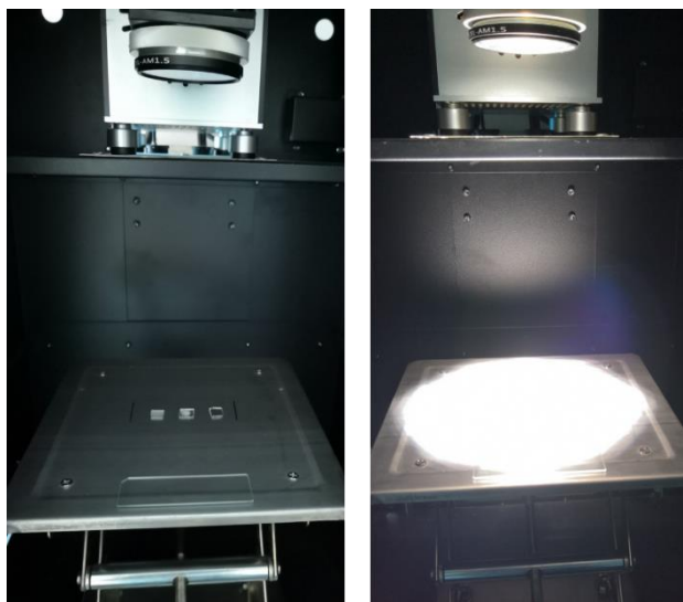
Figure S7. Photos of the simulated sunlight setup for light-to-thermal imaging tests.
