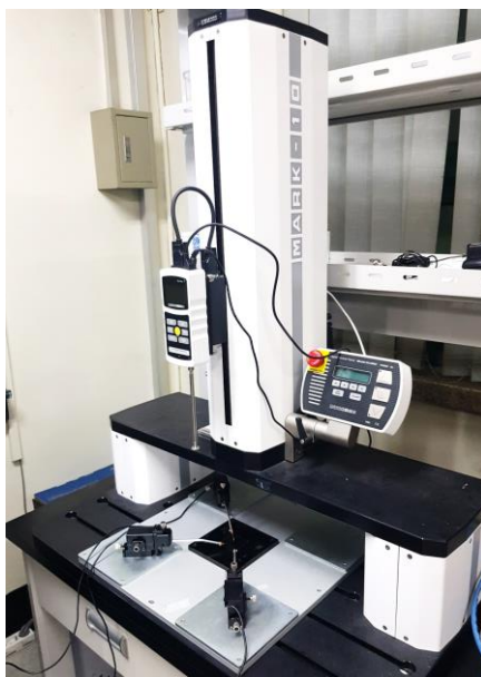
Figure S8. The experimental setup that consisted of a motorized z-axis stage (Mark-10 ESM303) and a force gauge (Mark-10 M7-20).
