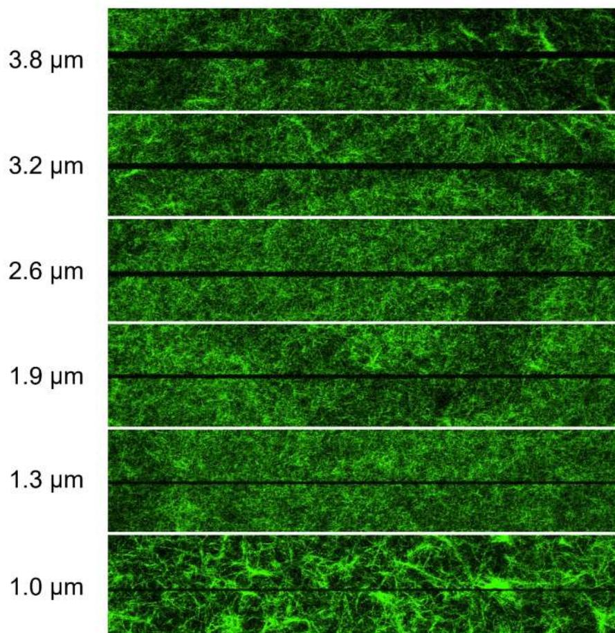
**Figure S1: Ablation resolution testing.** Channels with width ranging from 1.0  $\mu\text{m}$  to 3.8  $\mu\text{m}$  were ablated into collagen using a two-photon microscope, with settings as described in the main text, and visualized using second-harmonic generation imaging. The measured width of ablated channels corresponded precisely with the intended widths shown to the left of the figure.
