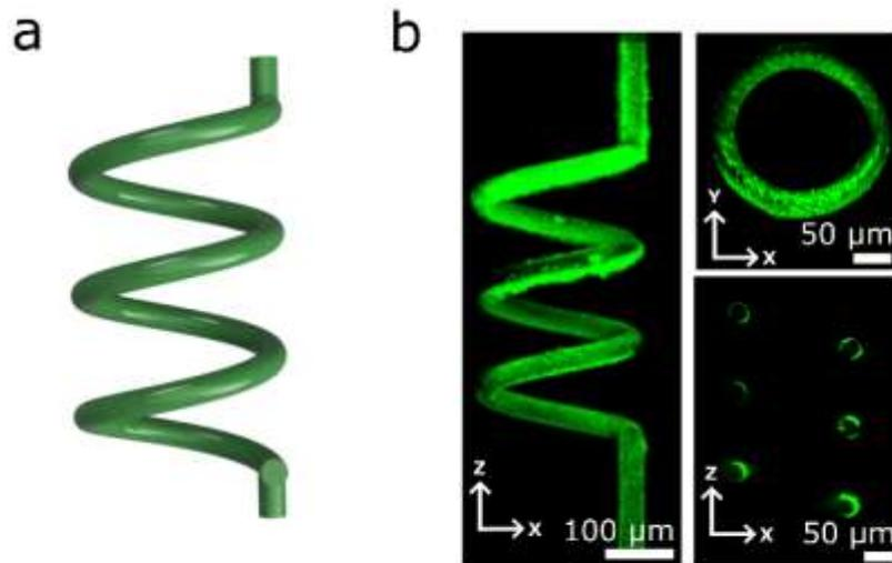
**Figure S2: Design and ablation of a perfusable helical structure.** **a**, Model CAD structure. **b**, Fluorescent bead perfusion of an ablated helical structure. XY projection (right, top) shows smooth circular curvature and an XZ optical section (right, bottom) demonstrates open, circular lumens.
