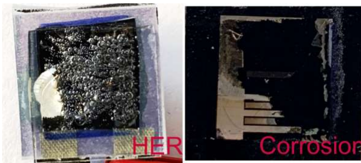
Figure S15. Image of hydrogen generation and corrosion of the Zn microanode.
