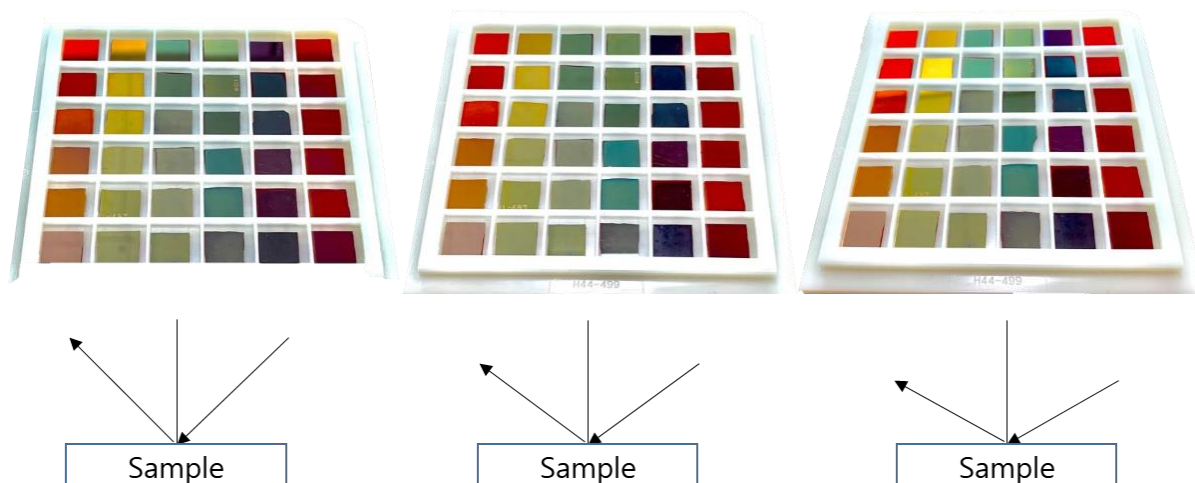
Figure S6. Incident angle-dependent color change. As the incident angle changes, the Fresnel equations yield different spectrum of the reflected light, although the color change is minimal for the angles used here.
