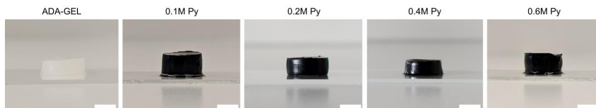
Figure S2. Hydrogel cylinders of ADA-GEL-PPy:PSS and ADA-GEL fabricated using different Py molarities. From left to right: ADA-GEL, 0.1M Py, 0.2M Py, 0.4M Py, and 0.6M Py. Scale bars: 5 mm.
