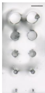
Figure S2: Minimum pore size in sintered Glassomer. The minimum achievable pore size was 14 \mu\text{m} (scale bar: 65 \mu\text{m} )
