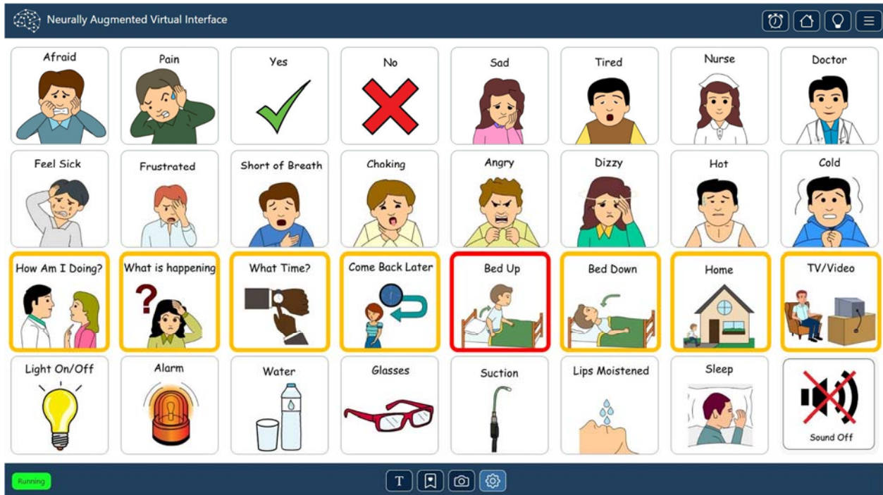
Supplementary Fig. 8 | User interface of communication board. The participant was instructed to select an experimenter-cued graphical button from a 4x8 grid by timing his brain-clicks to the appropriate highlighted row or column during the switch-scanning cycle. Switch-scanning started by sequentially highlighting each row in green (not shown) for 1 s until the participant brain-clicked on the row containing the cued button. Once a row was selected, all eight buttons in that row became outlined in gold and then each column was sequentially highlighted for 1 s in red. Once the participant selected a button by brain-clicking, the button became green for 1 s before the switch-scanning process was reset at row 1 and the participant received another cue.
