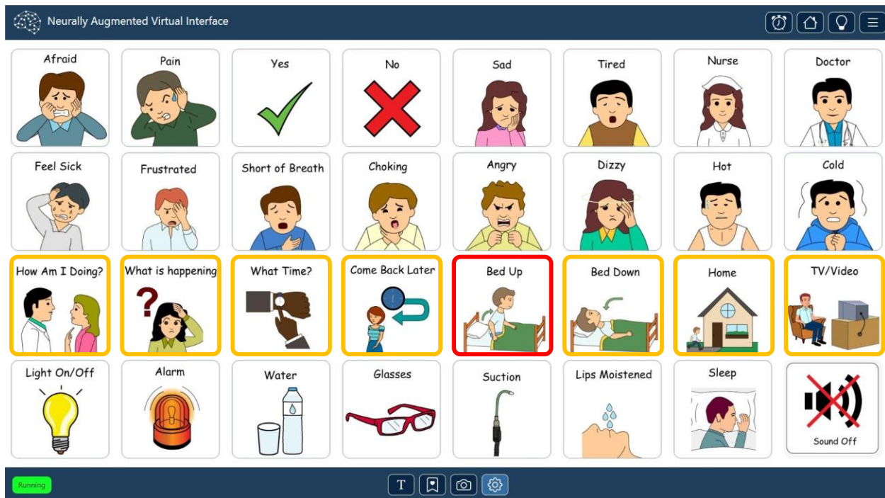
Supplementary Fig. 8 | User interface of communication board. The participant was instructed to select an experimenter-cued graphical button from a 4x8 grid by timing his clicks to the appropriate highlighted row or column during the switch scanning cycle. Switch scanning started by sequentially highlighting each row in green (not shown) for 1.5 s until the participant clicked on the row containing the cued button. Once a row was selected, all eight buttons in that row became outlined in yellow and then each column was sequentially highlighted for 1 s in red. Once the participant selected a button by clicking, the button became green for 1 s before the switch scanning process was reset at the first row and the participant received another cue. Pictograms were obtained from https://communicationboard.io/ 8 and ARASAAC ( https://arasaac.org/ ) 9 .
