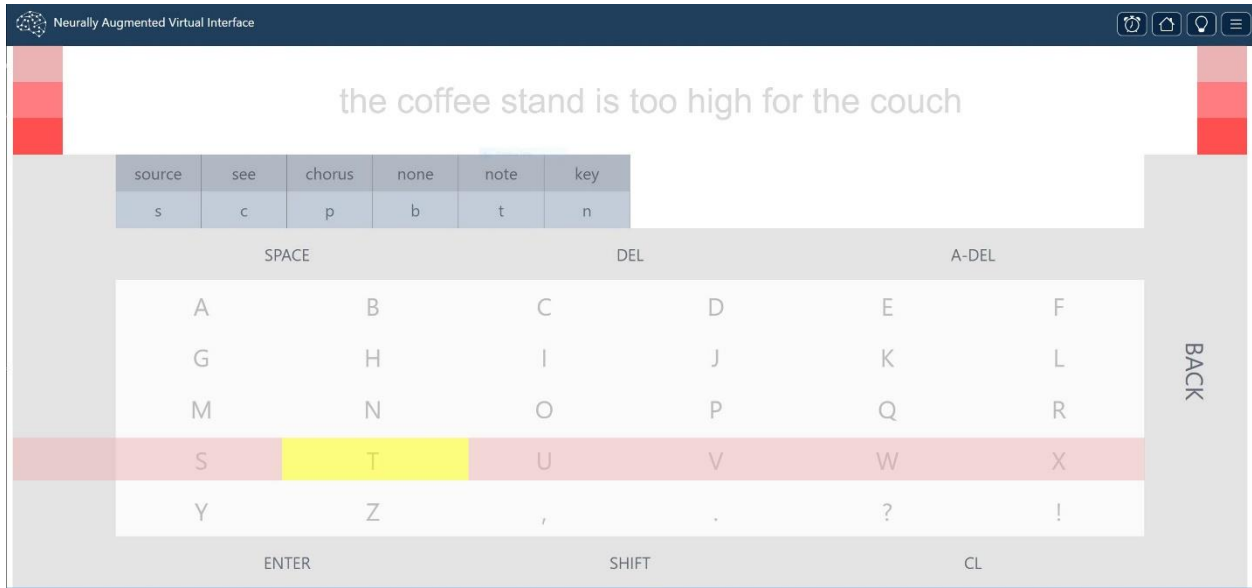
Supplementary Fig. 9 | User interface of switch scanning speller application. The participant was instructed to spell the sentence prompt (pale gray text) by timing his clicks to the appropriate highlighted row or column during the switch scanning cycle. The switch scanning process started by sequentially highlighting the three red pre-selection markers on either side of the sentence, where each highlight lasted 1 s. This was to allow the participant a brief preparation period in case he wanted to select row 1. Rows 1-8 were then scanned sequentially until the participant clicked on the row containing the appropriate letter or word. Rows 1 and 2 displayed the language model's most likely words and letters based on what the participant had already spelled. Row 3 allowed the participant to add a space, delete a letter or space, or delete an autocompleted word or letter (SPACE, DEL, and A-DEL keys, respectively). Rows 4-8 contained all alphabetical letters (and some grammatical symbols) in case the desired letter was not suggested in Row 2. Once a row was selected, the gray pre-selection column on the left was highlighted in yellow for 1 s to allow the participant a brief preparation period in case he wanted to select column 1. Buttons in the selected row were then sequentially highlighted in yellow for 1 s. At the end of each sequence of column highlights, the BACK key was highlighted to allow the participant to exit the row if it was selected accidentally. Clicking on any button (which would highlight it green for 1 s) within any row would reset the switch scanning process to Row 1. The participant finalized the sentence by selecting the ENTER button in Row 8. The SHIFT (for letter capitalization) and CL buttons (for erasing the spelled words) were functional but not used during the testing sessions. If the participant had not selected any of the eight rows, the switch scanning process was reset to Row 1.
