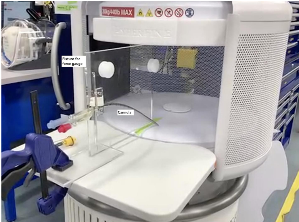
Supplemental Figure 1: Fixture with a cannula attached to ULF-pMRI scanner (spring gauge unattached).
