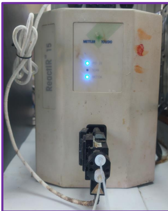
Figure S4. Actual photograph of ReactIR 15 flow cell setup.
