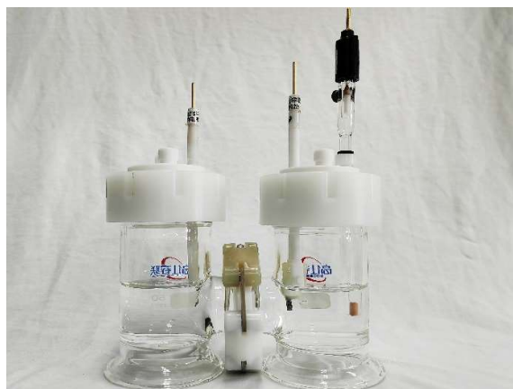
Fig. S33 The digital images of H-type electrolytic cell.
