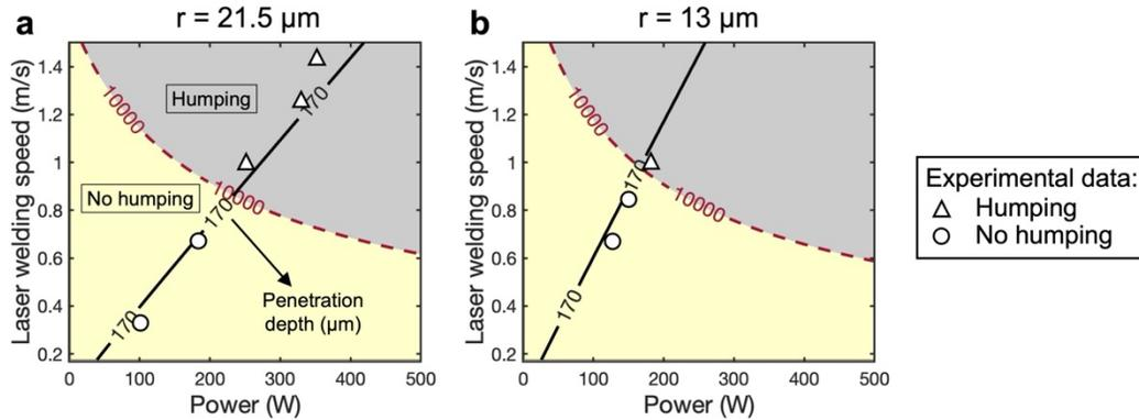
**Supplementary Fig. 5 Experimental validation of onset threshold of humping predicted by dimensionless humping index ( $\pi_h$ )**
