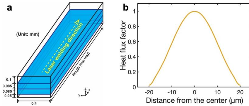
**Supplementary Fig. 3 CFD simulation setup**
