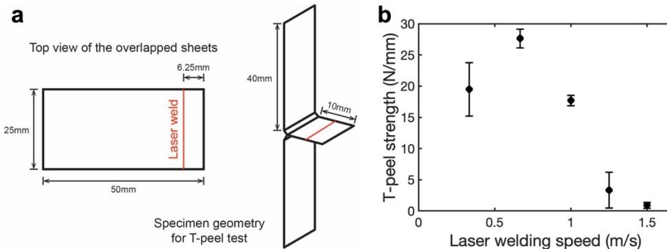
**Supplementary Fig. 2: T-peel strengths of laser welds**
