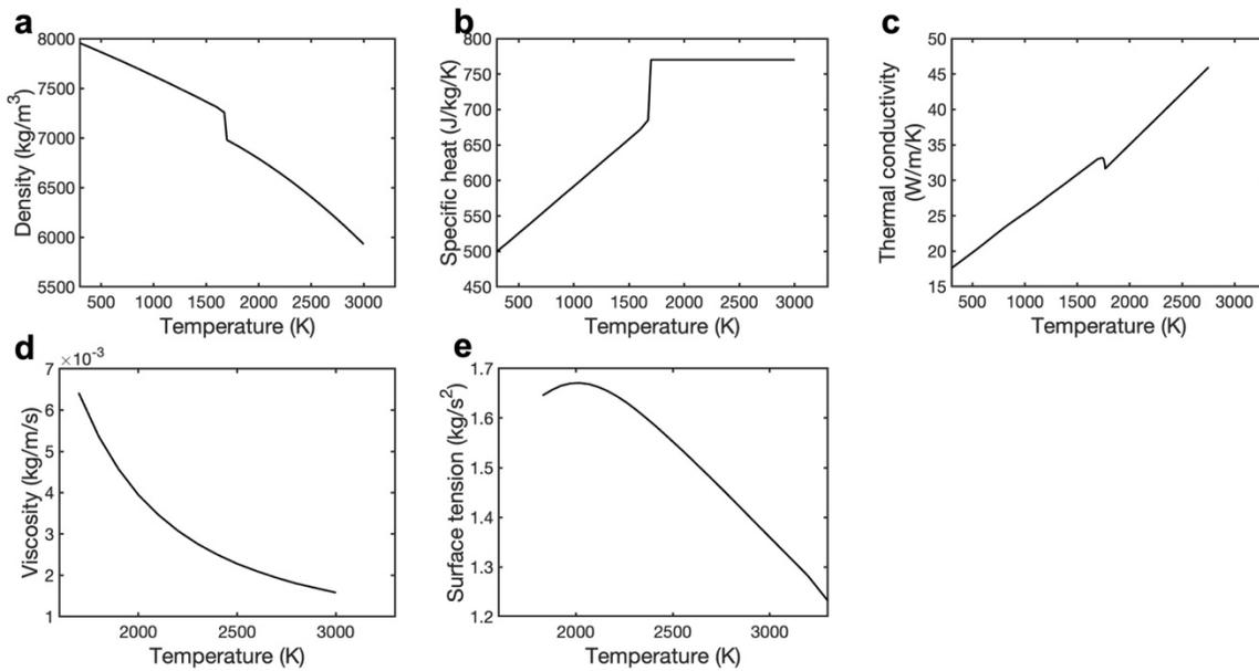
**Supplementary Fig. 4 Thermophysical properties of stainless steel**
