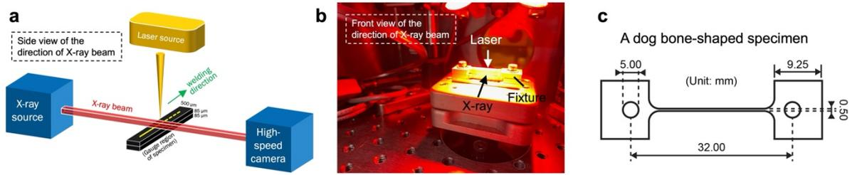
**Supplementary Fig. 1: Experimental setup of in situ high-speed synchrotron X-ray imaging at ANL**
