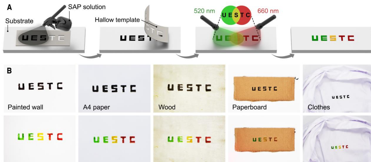
Fig. S7. Color-changing behavior of SAP coatings on different surfaces. (A) Schematic illustration of the mask-assisted spray-coating process and irradiation method of green light (520 nm), red light (660 nm) and mixed yellow light. (B) Images of SAP coating on rough surfaces (painted wall, A4 paper, wood, paperboard and clothes), images of the above surfaces irradiated by green light(520 nm), red light(660 nm) and mixed yellow light.
