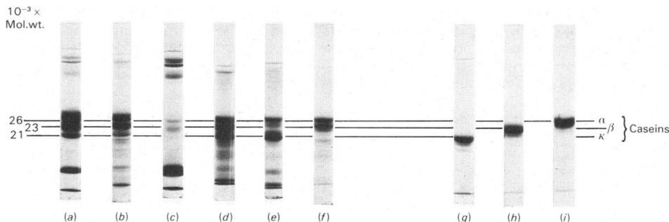
**Fig. 2. Analysis of the zinc-binding proteins of cow's milk by electrophoresis on SDS/10%-polyacrylamide gels**
