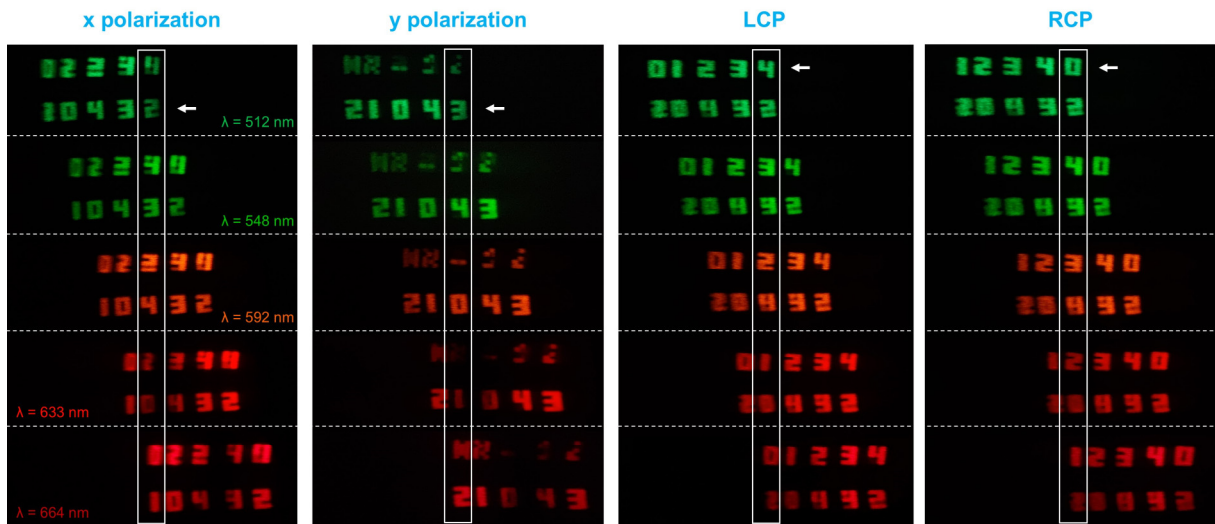
Supplementary Figure 18. Experimentally captured vectorial holographic images. The experimentally observed vectorial holographic images on the screen at different incident wavelengths and detected polarization states. The white rectangle indicates the designed observation angle of 40^\circ , while the white arrow represents the row corresponding to the designed polarization channel.
