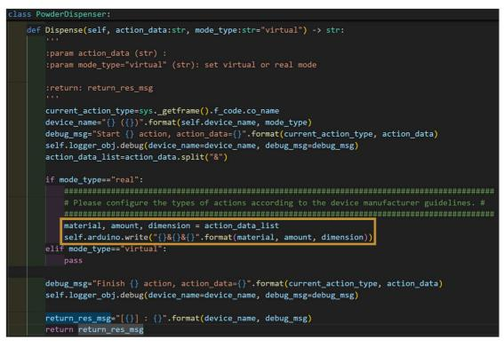
For example, in the case of a powder dispenser made with Arduino, the coding that entered material name, amount, and dimension is already done. Therefore, the 'action\_data\_list' should include these three information, and should be included diverse information depending on device. Use the 'write' function of 'self.arduino', defined in the constructor function, to execute the 'Dispense' function of the powder dispenser made with Arduino.
