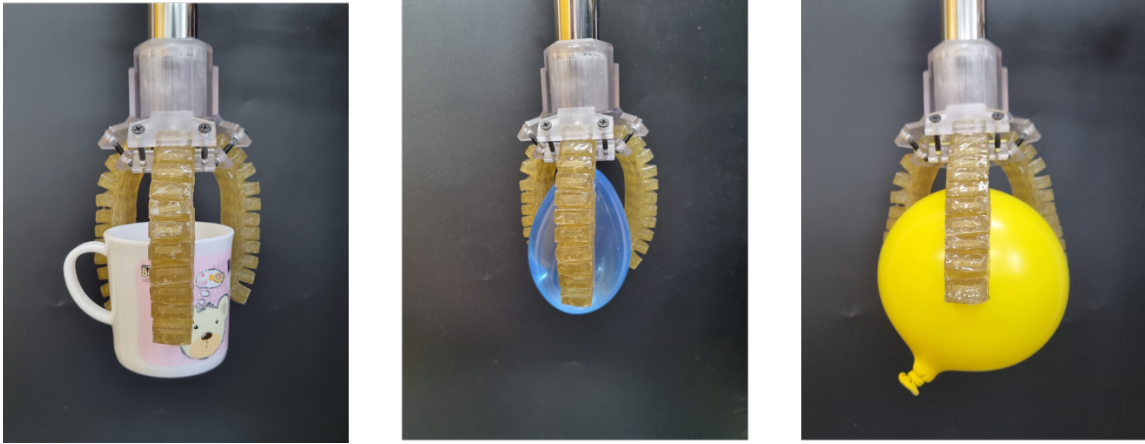
Supplementary Figure 29. Bending soft pneumatic actuator for soft gripper applications.
