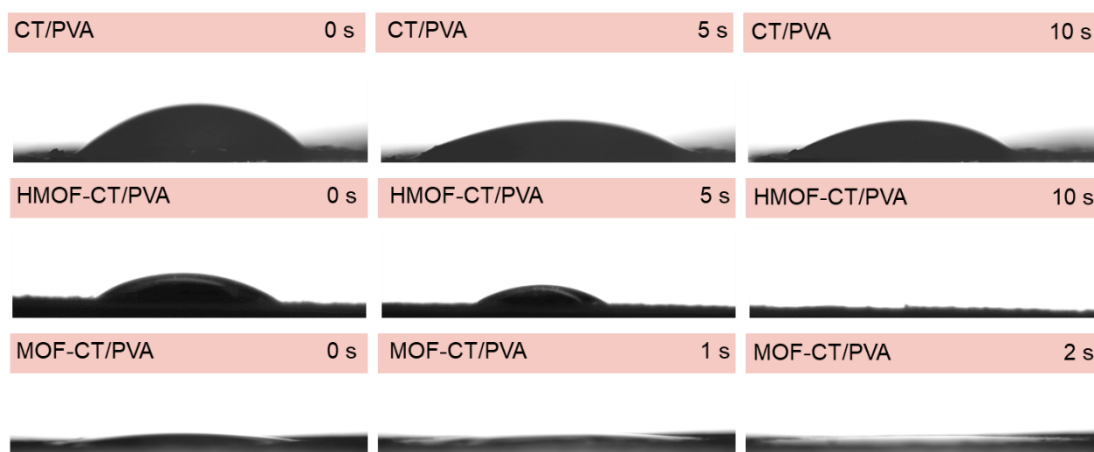
Supplementary Fig. 12. Changes in water contact angle of CT/PVA, HMOF-CT/PVA, and MOF-CT/PVA over time.
