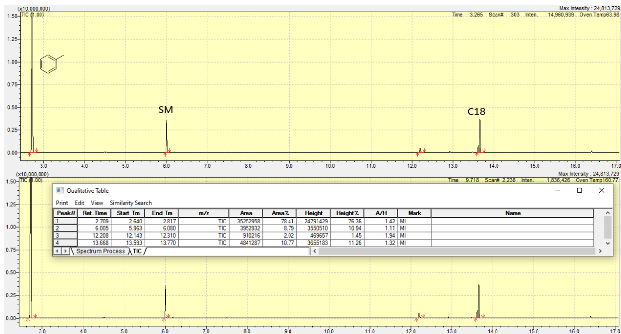
Figure S22. Entry 10. 240-minute aliquot of 2.5 mol % boric acid 5 mol % Grubbs 1 reaction. Shouldered peak at 12.2 minutes is a phthalate impurity on the GC/MS column.
