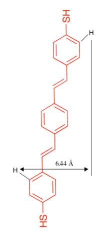
Molecular width = 6.44 Å + (2 \* 1.0 Å)= 8.44 ÅMolecular thickness = 2 \* 1.77 Å = 3.54 ÅMolecular area = 8.44 Å \* 3.54 Å=  $30 \text{ Å}^2$
