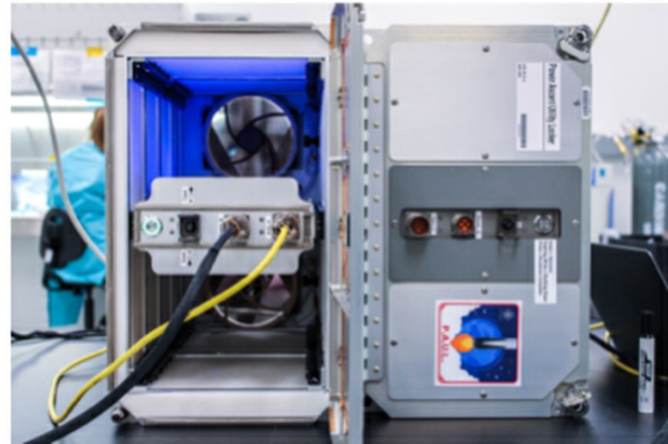
Supplementary Figure 1: CubeLab (top and bottom-left) facility that will house the vibrational bioreactor and the biological samples. The PAUL (top and bottom-right) facility designed to house and provide mechanical, electrical, and network interface from the outside
