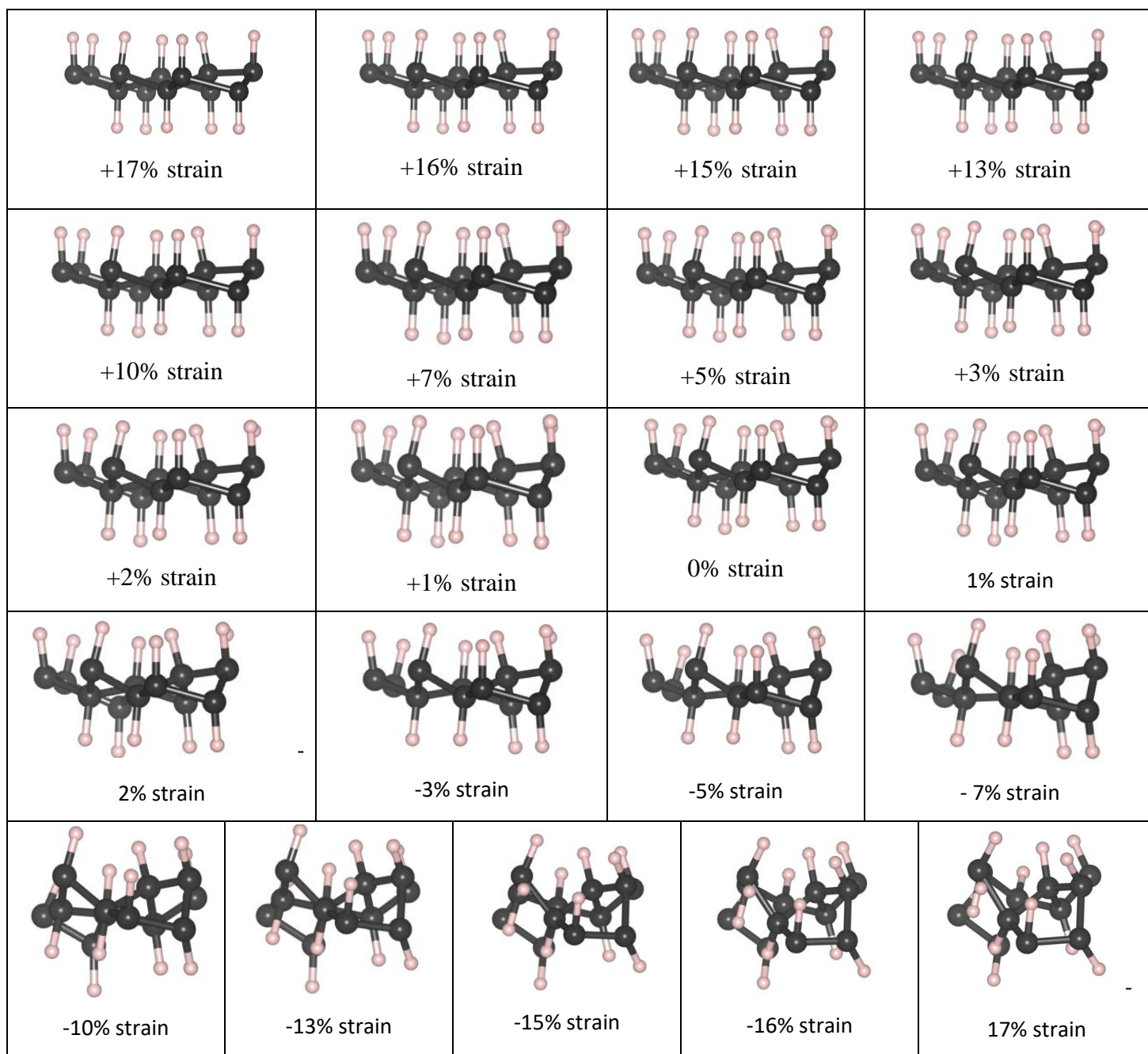
Figure 11: Side view of the relaxed unit cell of \psi -graphane at different strain levels.
