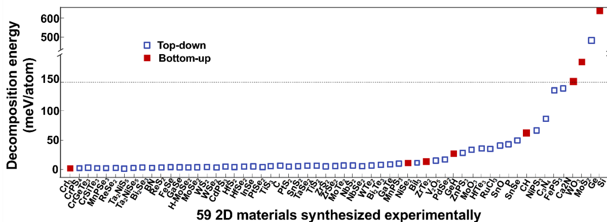
Figure S5. The decomposition energy of 59 experimentally obtained 2D materials. The blue open and the red solid blocks are the decomposition energies of 2D materials generated using top-down and bottom-up methods, respectively.
