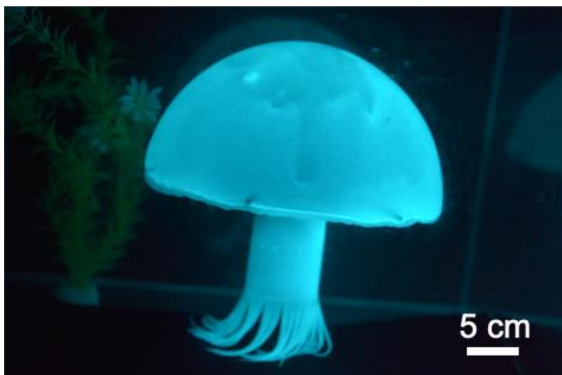
Fig. S1. The assembled Jellyfish powered by ZnBr 2 flow battery illuminated in darkness.
