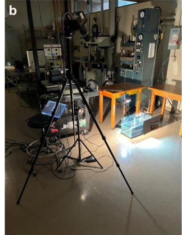
Fig. S7. Experimental setup of high-speed capture. (a) Schematic. (b) Optical image.
