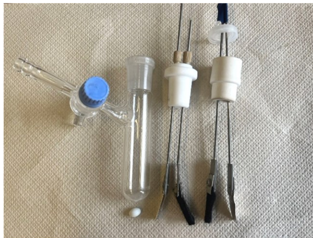
Figure S1. Picture of the electrochemical cell, stirring bar, and teflon cap with a graphite felt (GF) anode and a platinum (Pt) cathode
