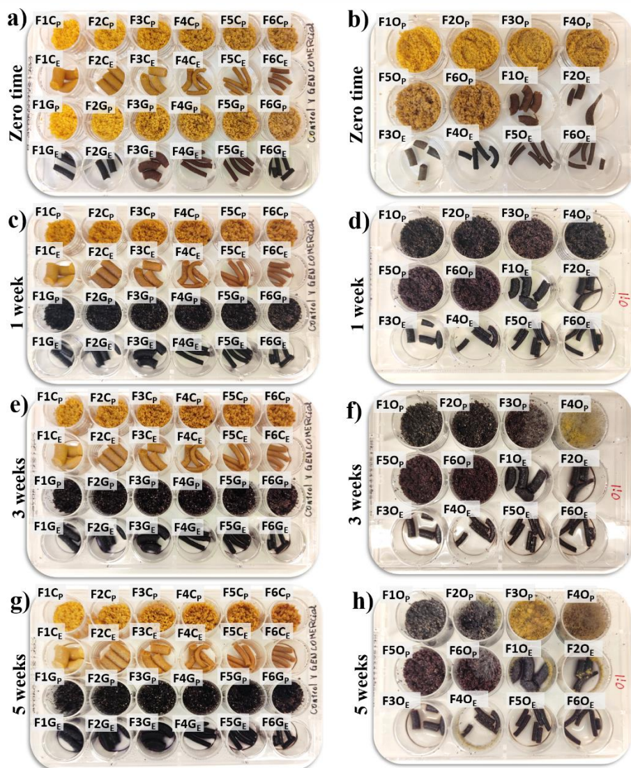
Figure S7. Mold resistance of the formulations developed in powder form (Pre-extruded, p ) and the extruded formulations ( E ) for the control samples, with genipin (a, c, e and g) and genipap oil (b, d, f, and h) as a function of time. The mould resistance was explored by exposing the powders and their extrudates to 100% humidity at 25 °C.
