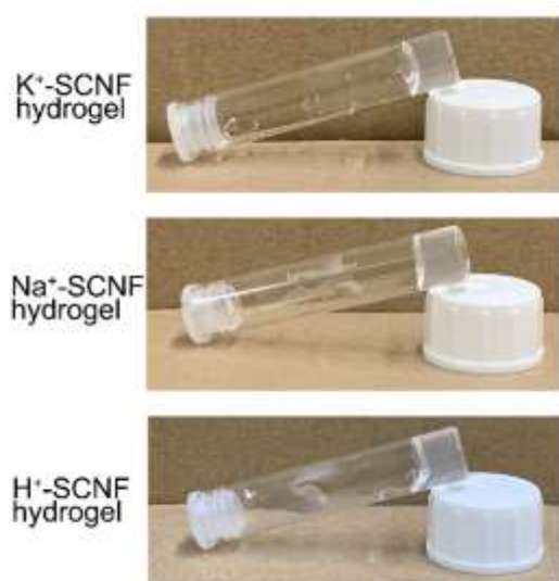
Figure S7. Digital photographs of K^+ -SCNF, Na^+ -SCNF and H^+ -SCNF hydrogels. The concentration of K^+ , Na^+ and H^+ is 0.1 M.
