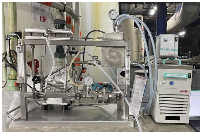
Figure S2. Photograph of the bench-top RO lab plant used in this work.
