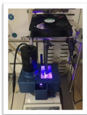
Figure S12. Kessil lamp set-up for the quantum yield determination
