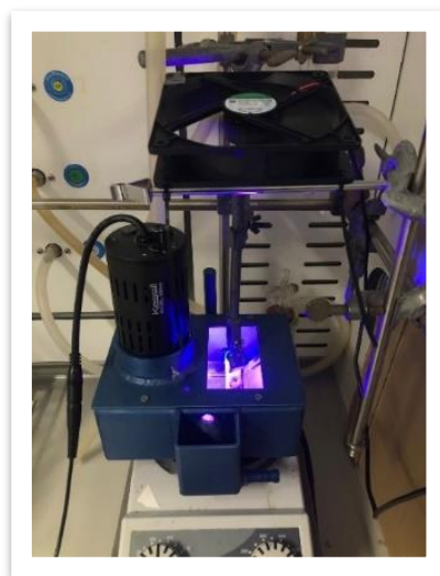
Figure S3. Reaction setup using PhotoRedOx Box TC™ reactor with 390 nm Kessil lamp.
