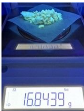
Figure S2. Fluorescent photograph of purified sulfur quantum dots for a patch of experiment.
