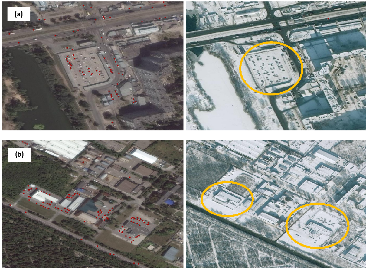
Figure S20: Illustrative example from Dnipro city to show the effect of snow on the detectability of cars. Both panels highlight two distinct commercial areas (a, b), with left and right panels showing the detected cars (red squares) on a summer and winter day, respectively. In the presence of snow (right panels), cars covered by snow remained undetected due to the reduced contrast. The orange circles in the right-side panels highlight the areas where cars remained largely undetected. Satellite images © 2019–2023 Maxar Technologies.
