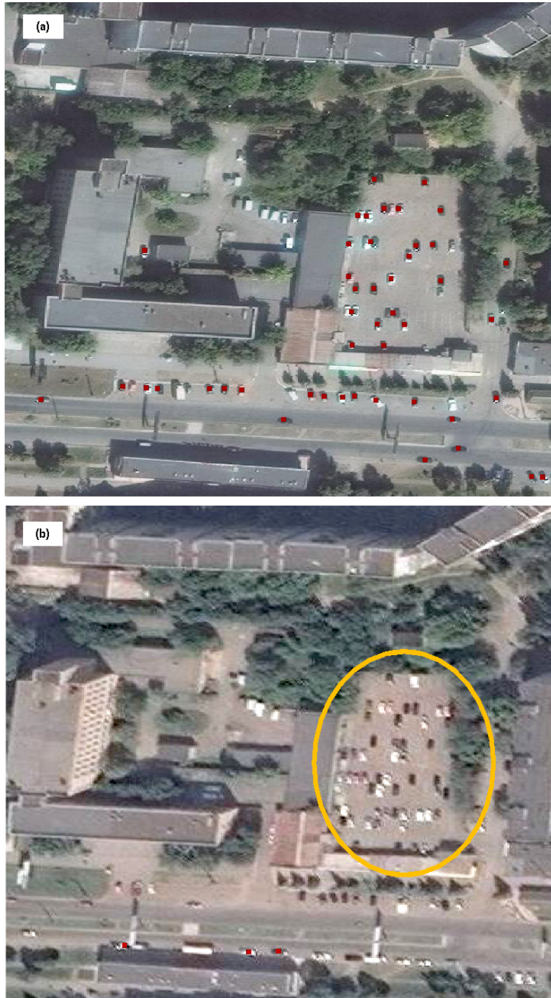
Figure S19: Illustrative example from Alchevsk city on the effect of image resolution on car detection (marked as red squares in the images). The two panels shows a parking lot in front of a post office, whereby the Convolutional Neural Network (CNN) model detects visibly more cars in the higher- resolution image (0.3 m GSD; panel (a)) than in the lower-resolution image (0.5 m GSD; panel (b)). Note that both images were taken on similar time and dates (a = 12.09.2019 08:55 UTC, b = 24.08.2019 08:22 UTC), as well as had similar imagery features: off-Nadir angle (a = 17.56^\circ , b = 24.14^\circ ), sun elevation (a = 45.58^\circ , b = 50.42^\circ ). The orange circle in panel (b) highlights the area where cars remained largely undetected. Satellite images © 2019–2023 Maxar Technologies.
