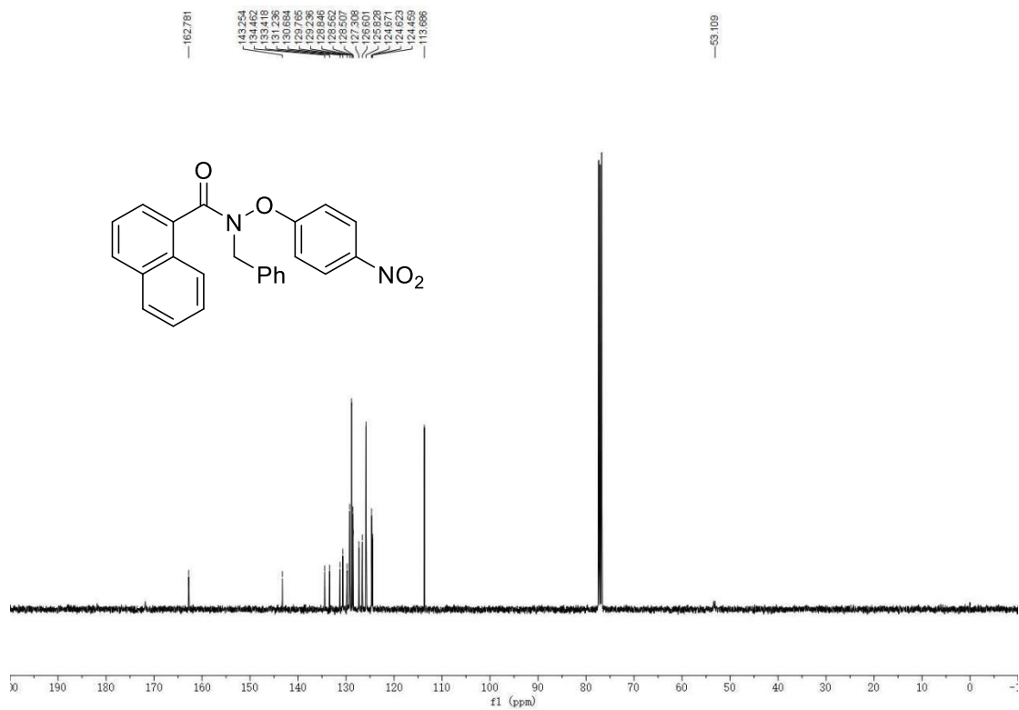
Figure S32. ^{13}\text{C} NMR spectra (100 MHz, Chloroform- d ) of N -benzyl- N -(4-nitrophenoxy)-1-naphthamide ( 1d )
