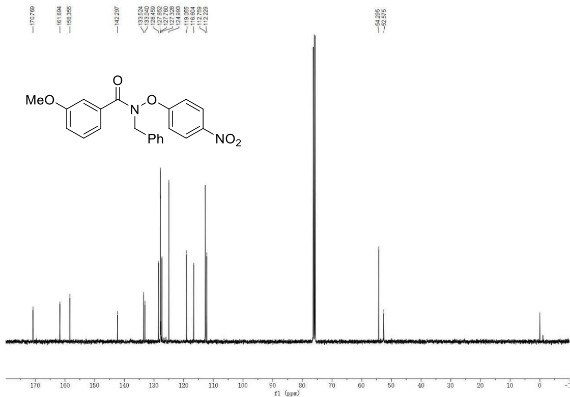
Figure S27. ^{13}\text{C} NMR spectra (100 MHz, Chloroform- d ) of N -benzyl-3-methoxy- N -(4-nitrophenoxy)benzamide (1b)
