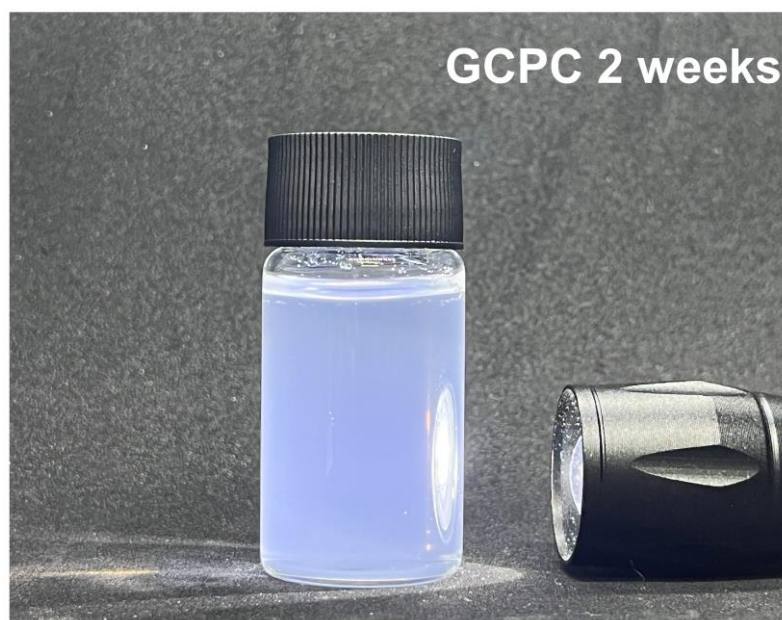
Fig. R6. The digital image of the light scattering of the glycerol-diluted GCPC after storage for 2 weeks.
