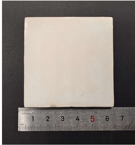
Supplementary Figure 23 | Photograph of RCWSM. The sample size is about 60 mm × 60 mm × 4 mm.
