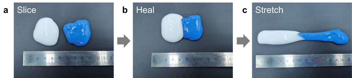
Figure R3. Predesigned hydrogel of rigid cavity layer. Self-healing process of PVA/qCNF/GB hydrogel, including as slices before healing (a), rapid healing behavior while occurring to sufficient interfacial contact (b), and the robust combination demonstrated under the stretch (c).
