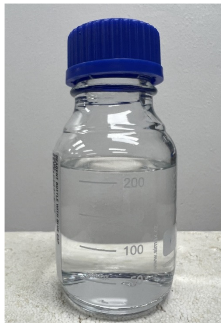
Fig. S64. Digital photograph of the product obtained after 100 h of operation, consisting of a mixture of cyclohexane and chlorocyclohexane. Note: the aqueous electrolyte was removed using a separating funnel. The 100 h measurement was separated into 25 cycles, with 4 h in each cycle. Every cycle uses 90 ml of 1 M KCl electrolyte and 10 ml of cyclohexane.
