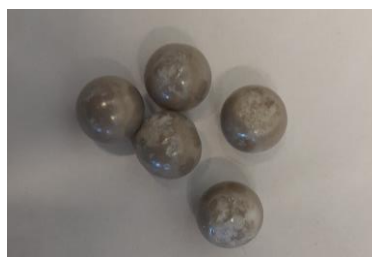
Fig. S8. Photograph of 5 damaged \text{ZrO}_2 grinding spheres (10 mm diameter) after repeated milling at 35 Hz with low plastic filling degrees of model PP.
