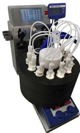
Supplementary Figure 1. The photoreaction instrument: WATTCAS_WP-TEC-1020LC
