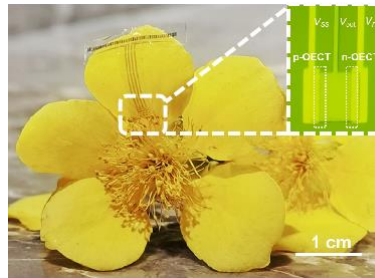
746 Supplementary Fig. 52 Photograph and magnified microscope image of the thin and flexible 747 inverters. Attached to a fragile petal.
