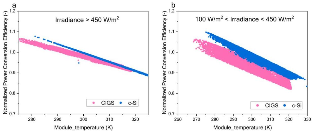
Supplementary figure 3: Normalized power conversion efficiency plotted for different irradiance regimes. a) Incident irradiance  $> 450 \text{ W/m}^2$ , b)  $100 \text{ W/m}^2 < \text{incident irradiance} < 450 \text{ W/m}^2$ . The data points is cumulative of simulation data from the PV integrated sound barrier system in Kuwait and Belgian climate.
