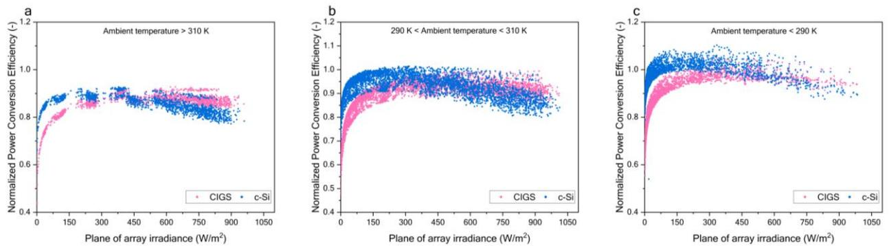
Supplementary figure 4: Low-light performance of c-Si and CIGS technology. The top row figure panels compares nPCE for c-Si (blue) and CIGS (pink) technology for ambient temperatures a) less than 290 K, b) In between 290 K and 310 K, and c) greater than 310 K. The data points is cumulative of simulation data from the rack mounted PV system in Kuwait and Belgian climate.
