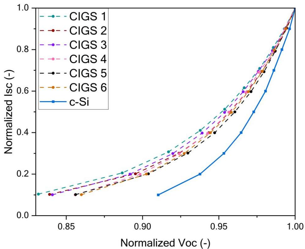
Supplementary figure 5: Measured Voc-Isc behaviour of different CIGS modules (dotted lines) compared with c-Si PERC module (Solid line)
