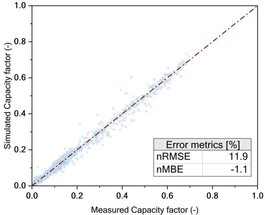
Supplementary figure 2: Simulated capacity factor plotted against measured capacity factor for c-Si module. The markers indicate the simulated data points while the black solid line represents the ideal scenario where the simulation is equal to the measurements
